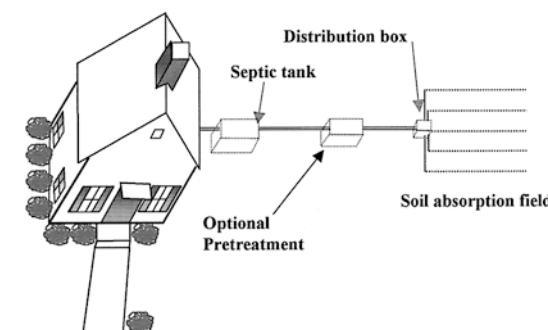
**Figure 1.** Schematic of on-site waste disposal system.
